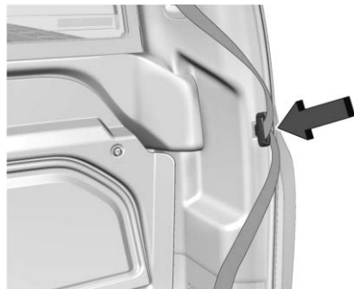
Midgate Lowered with Crossbar Attached
